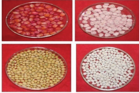
Uncoated and coated seeds with ZnO (<50 nm) @ 50 mg Zn/g seed of maize and soybean
