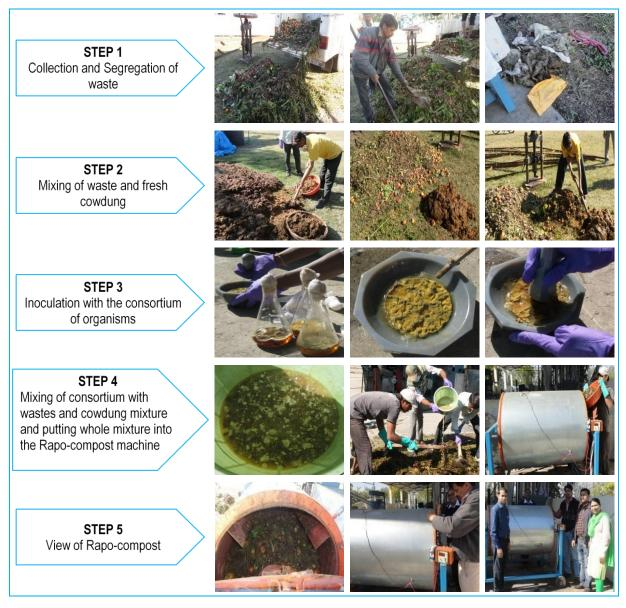
Figure 4. Schematic representation of Rapo-Composting Technology
