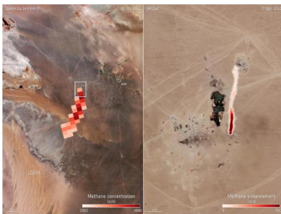
Figure 2: Methane super-emitter plumes detected in a cluster of detections at an oil exploitation site in Libya, as observed by Copernicus Sentinel-5P on 26 July 2021 (Source: Trio of Sentinel Satellites Map Methane Super-emitters, 2023)
