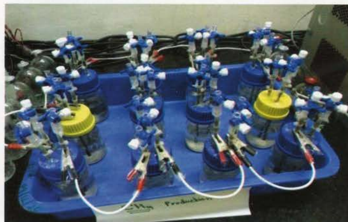
Biofuel cell: Cathode driven CH 4 production from CO 2
